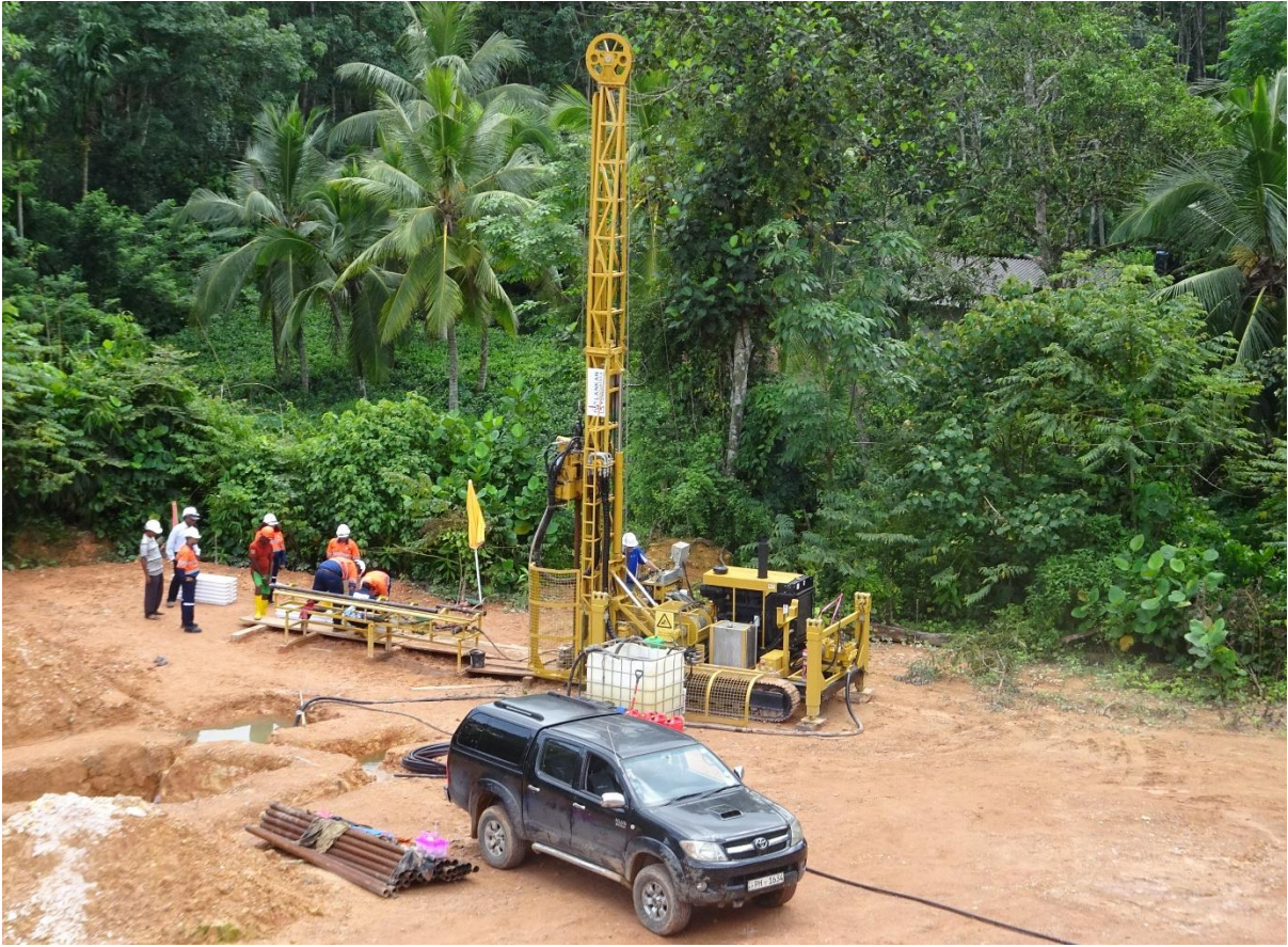
Figure 1. New Diamond Drill Rig working at Pathakada
